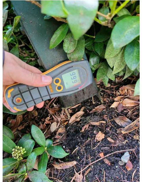
Elevated moisture reading
